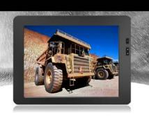
The slim-profile, lightweight DOD1200V2L all-weather monitor is housed in a billet aluminum enclosure with sealed connectors. Multiple mounting options allow for easy integration into confined spaces typically found in rugged industrial and mobile applications.
