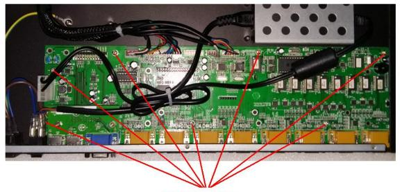
4. Unplug the selected terminal one by one and plug in to the new main board.
