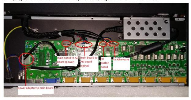
5. based on step  $3 \rightarrow 2 \rightarrow 1$  to screw back the main board, copper studs and rear cover.
