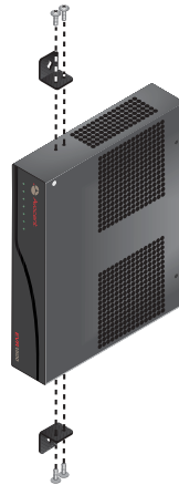
Figure 2.1: EVR1500 Environmental Monitor Appliance Wall Mounting Diagram
