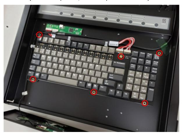
5. Disconnect wires from the touchpad and remove the screws that hold the touchpad in place.
