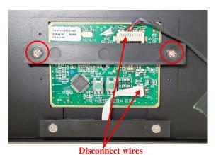
6. Reconnect wires and reassemble touchpad.
