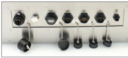
Power, USB, COM, VGA, LAN and Audio out
