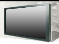
Front Water and dust Proof IP65/NEMA 4 with IP65 Solid Back housing except I/O. Industrial Chassis/Wall Mount Heavy Duty Metal Housing 27" LCD monitor, 1920x1080, 250 nits VGA + DVI + HDMI Input, Side OSD, with 1920x1080 with Projective Capacitive Touch (1-2mm) USB Controller, Internal power supply 100-240 VAC 50-60Hz
