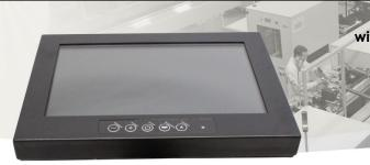
Wide 21.5" LCD monitor, 1920 x 1080, LED- 1000nits, Chassis design with 5 sides IP65 / AR glass / Front OSD Direct Control brightness from 5% to 100% + and - from the Front OSD membrane.
