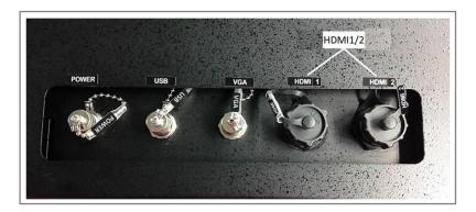
Power Input: 12VDC to 28VDC, 30 Watts
