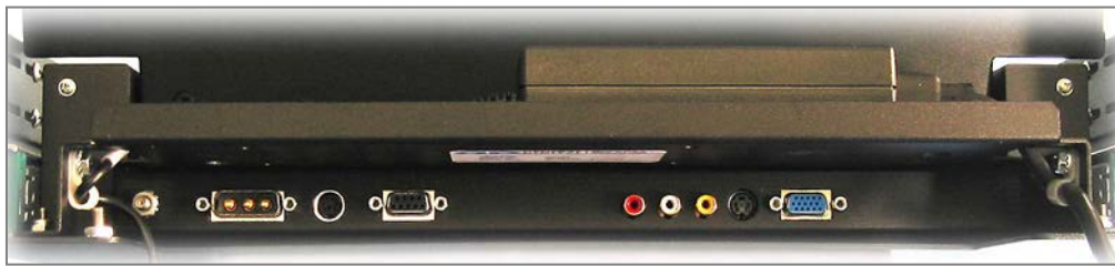
Rear view of 19" showing power supply and interface connectors
