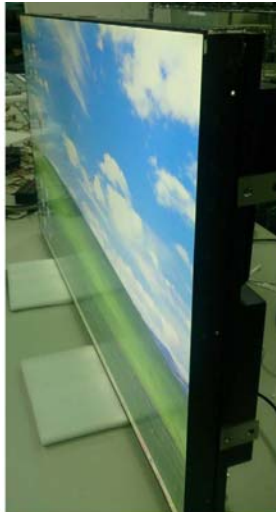
Special open frame chassis design for TV wall matrix
