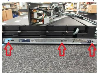
Step 4: Please release the screws on bottom chassis to replace the  $2^{nd}$  section of railway (3x each side)
