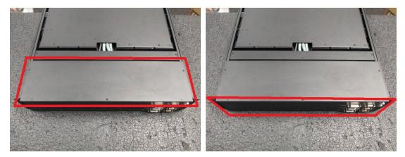
Step 2: Pull the drawer all the way out and release the locking mechanism to detach the drawer out of its bottom chassis, and please pull slowly and carefully to prevent the damage of falling drawer.
