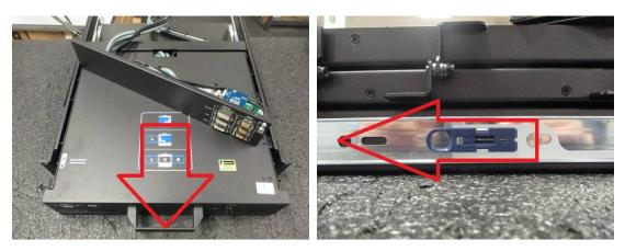
Step 3: Please release the screws on drawer to replace the 1<sup>st</sup> section of railway. (3x each side)
