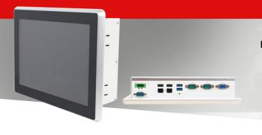
10.1" 400nits Panel PC IP65, NEMA 4 Rugged Protection, metal front bezel, 10 points projected capacitive Touchscreen. Intel Bay Trail-D J1900 2.GHz Quad Core CPU 4GB Memory, 32GB mSATA SSD No OS,- 1 \* 8bit GPIO
