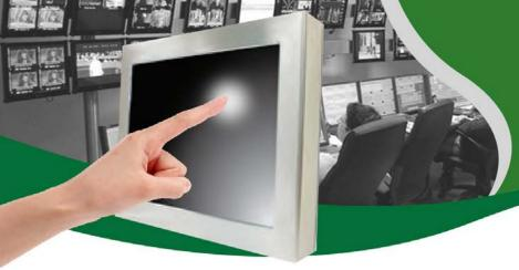
Fanless 21.5" Fully IP65 stainless steel panel PC with 5 resistive touch screen (Intel J1900 industrial main board + Fully IP65 stainless steel panel PC chassis (sliver) + DC in external
