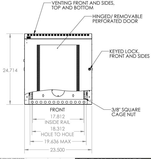
NOTE: 22.5 MAX RAIL TO RAIL 12.5 MIN RAIL TO RAIL
