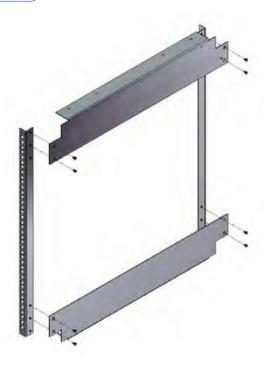
Place the left and right sides so that the mounting holes line up with the pre-drilled holes in the bottom of the work surface and attach with 4 screws.
