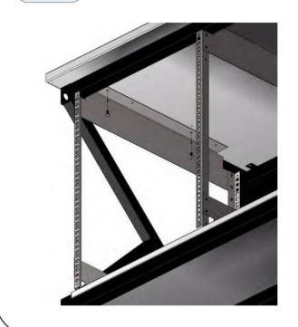
Attach the front and rear spacers with the 4 provided screws. If you would like added stability, you may use the provided wood screws to attach the bottom brackets directly to the bottom shelving.
