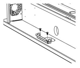
Secure the lock base just behind the grommet opening with the 1/4"-20 screws
