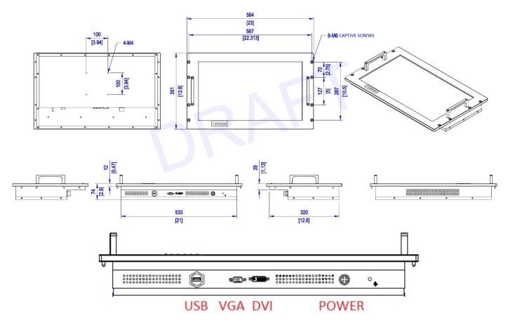
IO Ports: 1 x USB for Touch, 1 x VGA, 1 x DVI and 1 x Power Input for Display
