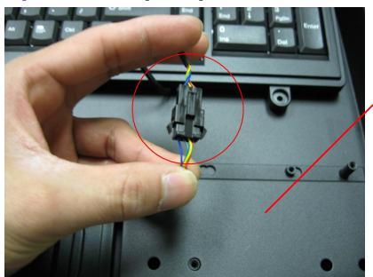
The 4-pin connector is under this cover
