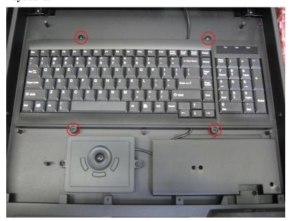
**Step 5b:** Remove 2 keyboard screws holder and then replace the defective mouse module.
