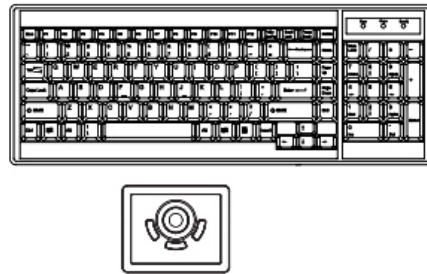
b keyboard integrated with trackball
