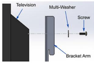
Step 2: Attach the two bracket arms to the back of the LCD monitor. Ensure that the bracket arms are attached vertically on the back of the screen.
