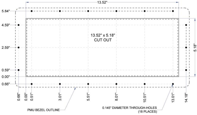
PMU BEZEL: ABS/Polycarbonate with 4-40 x 0.75" Metal Studs (18 Places)
