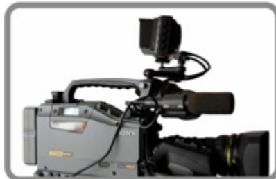
Working together with professional cameras, to get power from camera battery through a D-tap power cable.
