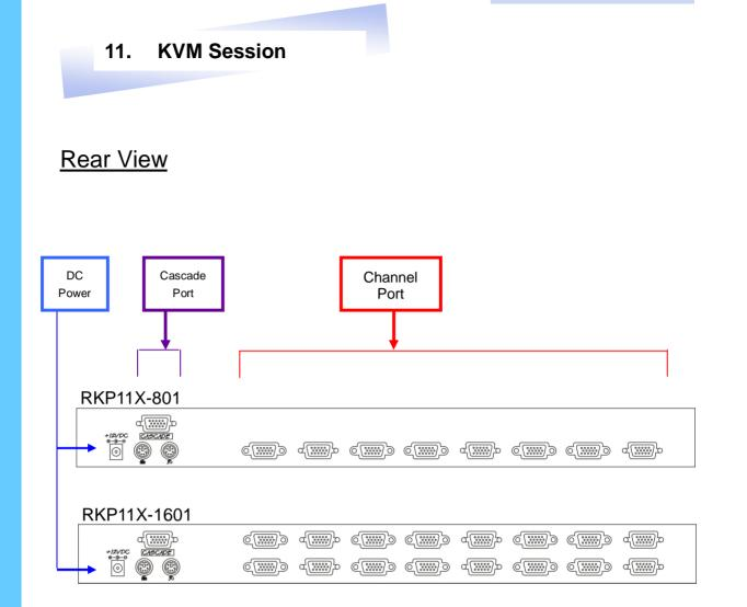
**DC Power** -connect to external 12V DC power adapter.
