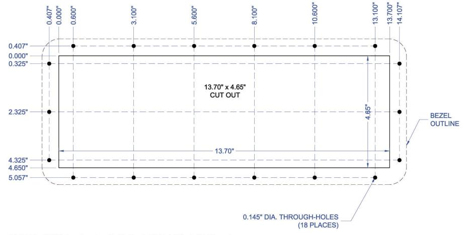
PM BEZEL: ABS/Polycarbonate with #4-40 x 0.50" Metal Studs (18 Places)
