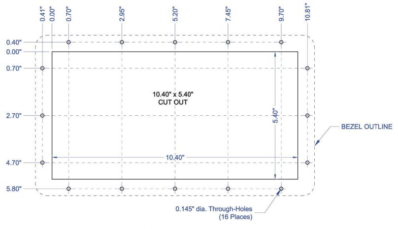
PMU BEZEL: ABS/Polycarbonate with #4-40 x 0.75" Metal Studs (16 Places)
