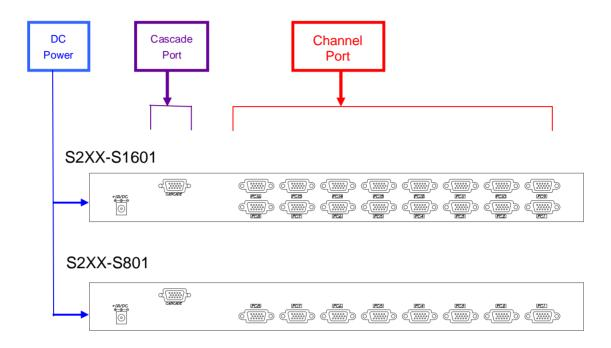
**DC Power** -connect to external 12V DC power adapter.
