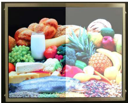
Figure 1. LCD module with bonded (L) and non-bonded (R) cover glass.
