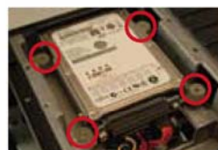
HDD install with Anti-shock buffer rubber enhances protection performance.
