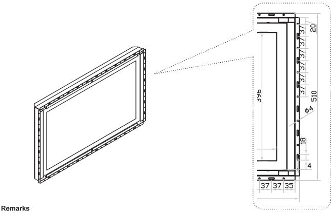
■ Hardware for fixing the LCD display is not provided
