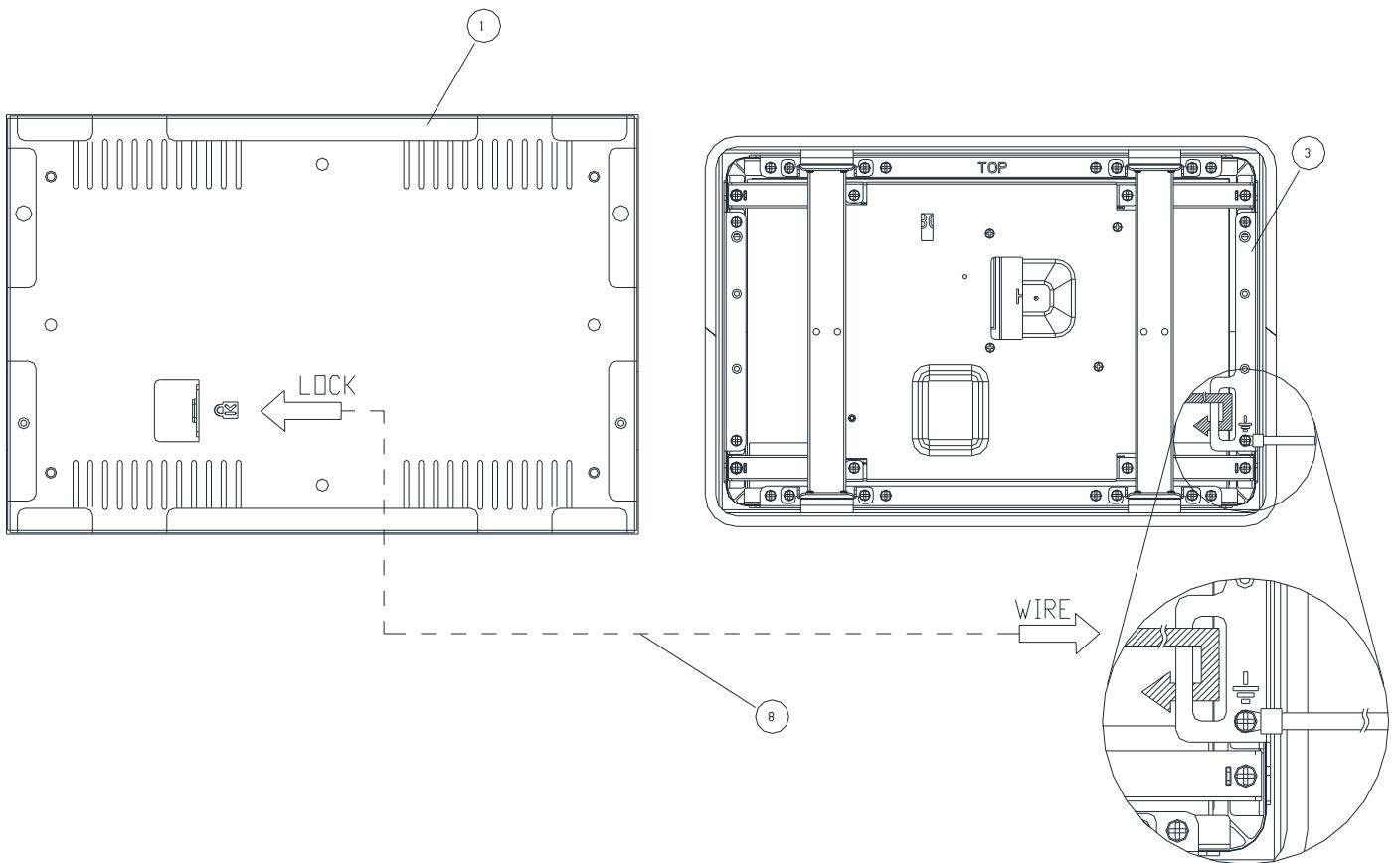
**Step5.** Wrap the Kensington lock (option) around the hole in the front bracket and attach the lock to the keyhole in the Wall box.
