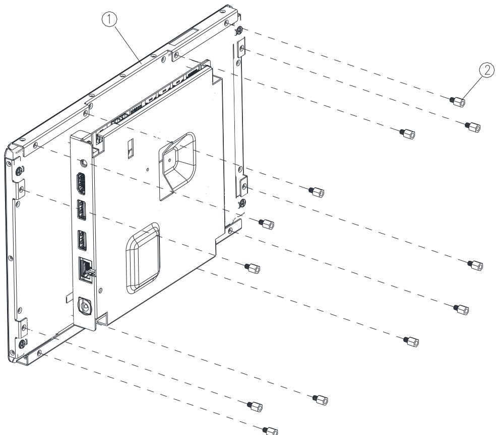
**Step1-1.** Locate brackets on both sides, matching the holes on the monitor.
