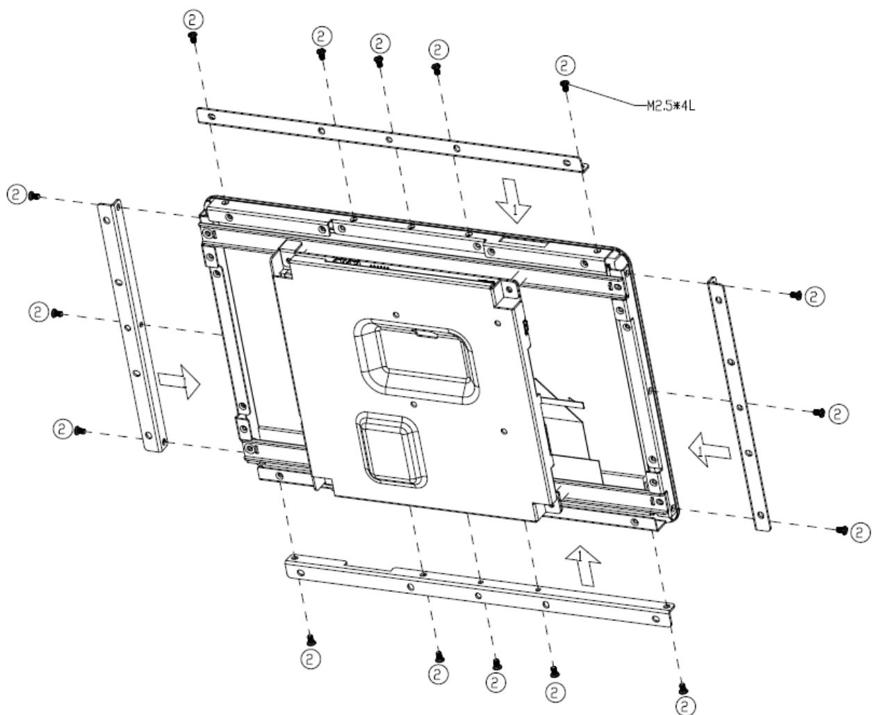
**Step1.** Locate brackets on both sides, matching the holes on the monitor.
