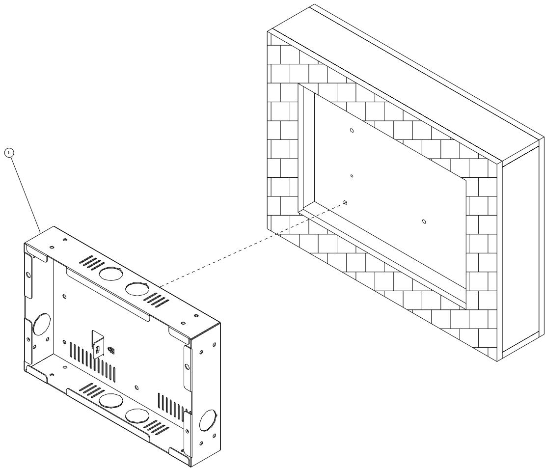
**Step1.** Fasten the screw on the wall.
