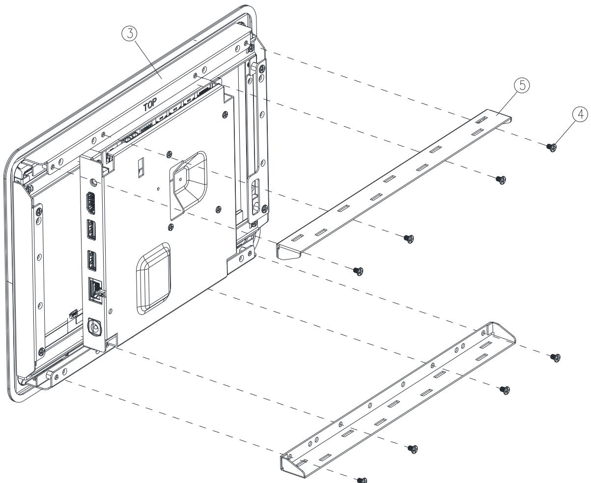
**Step3.** Insert and fasten 8 screws to secure Bracket T/B.
