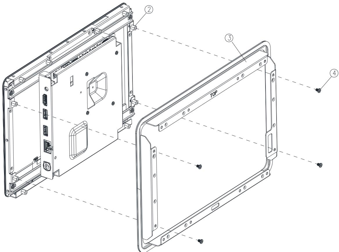
**Step2.** Insert and fasten 4 screws on each side of the monitor to secure Front bracket.
