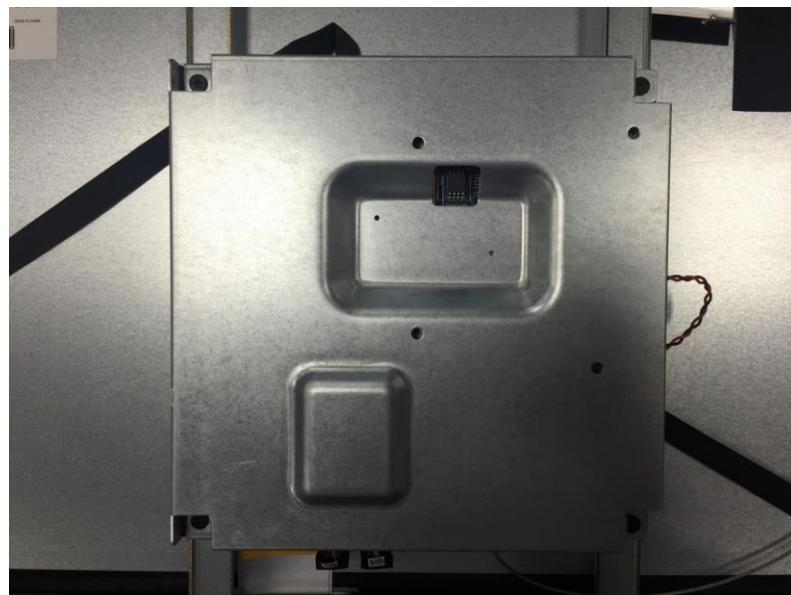
Remove all screws on shielding cover.
