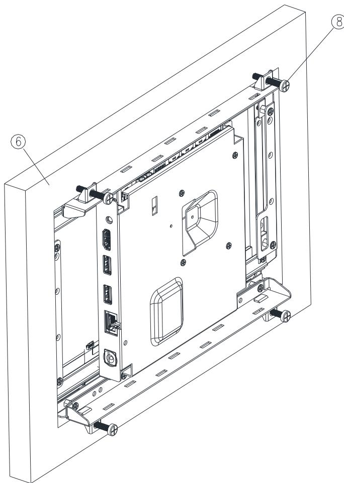
**Step6.** Insert and fasten 4 Panel mount screws to secure the module.
