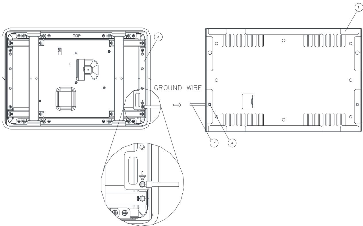
**Step4.** Insert and fasten 2 screws on Front bracket and Wall box of the monitor to secure Ground wire.
