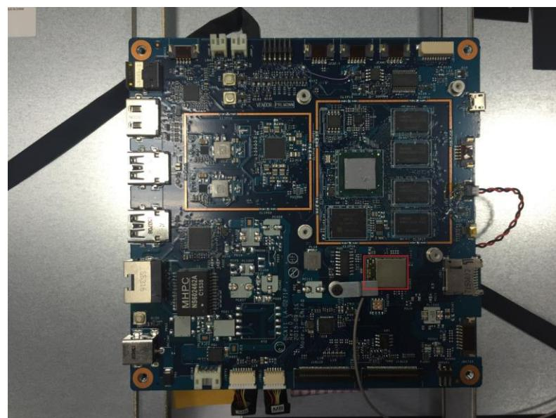
WiFi Module is located on MB underneath of the Shielding cover.
