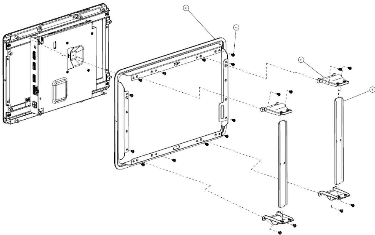
**Step3-1.** Insert and fasten 12 screws on each side of the monitor to secure Front bracket.
