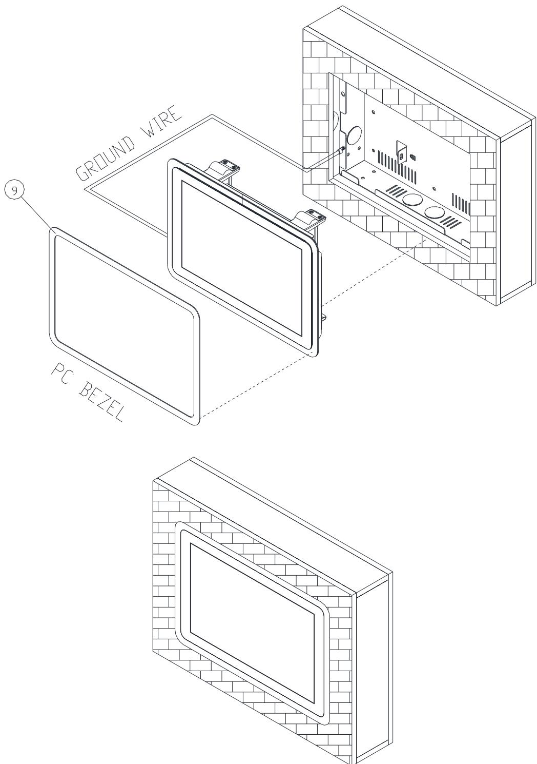
**Step6-1.** Insert the Ground wire and Kensington lock in the Wall box and Insert BCX11 10" Open frame into the wall.
