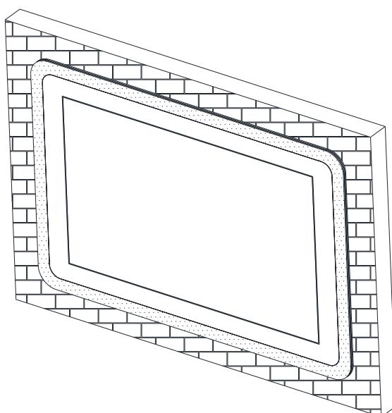
**Step7.** Paste the Decoration Plate on the Front bracket to complete installation.
