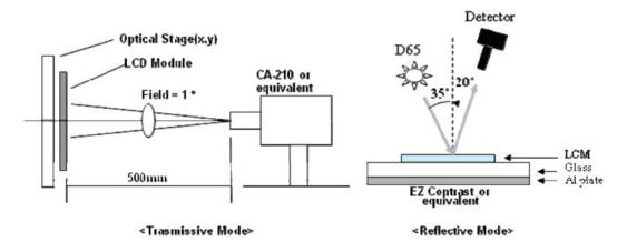
(Optical Characteristic Measurement Equipment and Method)
