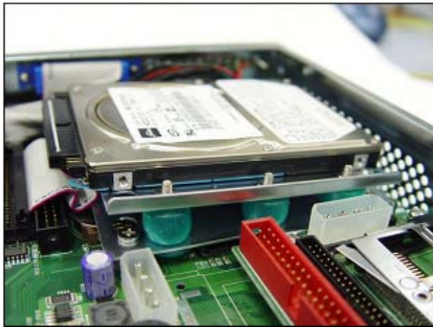
Hard Disk Anti-Vibration Kits for mobile solution
