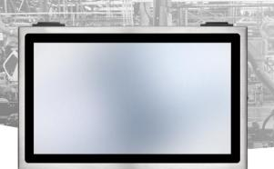
21.5" 1920x1080 Fanless -20 to 60C, Core i5-6200U2.3GHz Skylake WideTemp. SATA HDD, Wide temp. Resistive flat, Class 1 Division 2, ATEX Zone 2, and IECEx Certified Fanless Design with Highly Efficient Heat Dissipation for 60°C Environments Boots up with Self-Heating at -20°C, without a Heater
