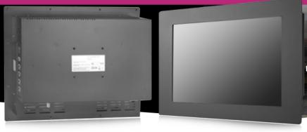
IP65 front Panel Mount (Metal-3mm), 24" LCD Monitor 1920 x 1080, 300 nits, VGA+DVI+HDMI, Side OSD, including rear screw/Clamp/VESA Mount with 5 Wire Resistive Touch Screen and USB Controller Integrated IP65 Front Panel
