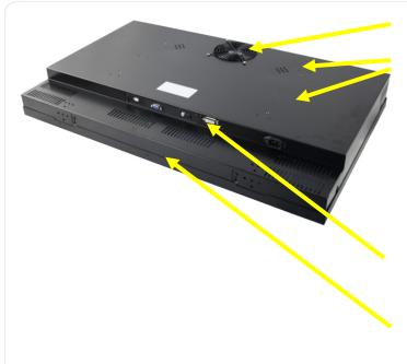
Ultra low speed/Noise fan for extra cooling (24" LCD or above) VESA Mounting Hole Pattern
