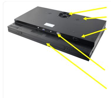
Ultra low speed/Noise fan for extra cooling (24" LCD or above)
