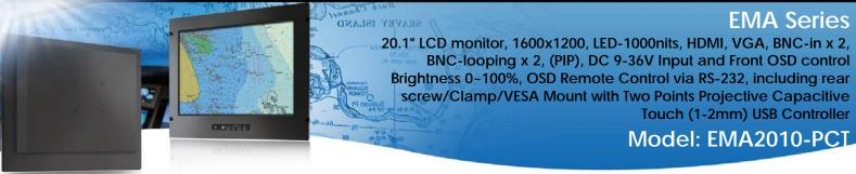
with Touchscreen With PIP, IP65 [Front], Wide Temp., Dimming, OSD Front Panel, Wide Voltage Input and High Brightness
