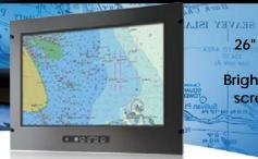
26" LCD monitor, 1366x768, LED-1000nits, HDMI, VGA, BNC-in x 2, BNC-looping x 2, (PIP), DC 9-36V Input and Front OSD control Brightness 0~100%, OSD Remote Control via RS-232, including rear screw/Clamp/VESA Mount with Two Points Projective Capacitive Touch (1-2mm) USB Controller
