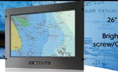
26" LCD monitor, 1366x768, LED-1000nits, HDMI, VGA, BNC-in x 2, BNC-looping x 2, (PIP), DC 9-36V Input and Front OSD control Brightness 0~100%, OSD Remote Control via RS-232, including rear screw/Clamp/VESA Mount with Capacitive Touch and USB Controller
