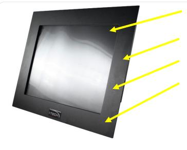
Metal 5mm Panel Mount for easy installation with stud mount and Clamps mount
