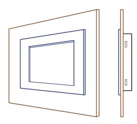
4-2. At the back side of the mounting wall, insert the mounting kits into the slide hole at the side bracket on the panel.
