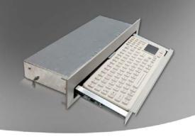
The YK9700E is an extremely small-footprint rackdrawer with an ergonomic 10-degree pullout drawer with magnetic lock. This rack drawer is ideal for use in harsh environments and its very shallow depth allows for storage behind the unit for crucial components such as a power source. The YK9700E-SK-97 comes standard with an SK-97-TP keyboard. Sealed to NEMA 4X specifications, the keyboard includes an integrated touchpad, 10-key numeric pad and rugged ABS polycarbonate case.
