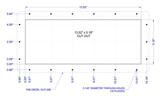
BEZEL: ABS/Polycarbonate with 4-40 x 0.75" Metal Studs (18 Places)
