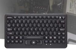
The Ymil-K600 offers a rugged keyboard and a rugged computer pointing device with an emergency key in one compact package. Meets MIL Standard 461-G. Ideal for military and public safety applications.
