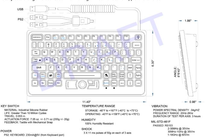
$3\;\text{X}\;\text{11}\;\text{ms}$  pulses of 50g on each of 3 axis
