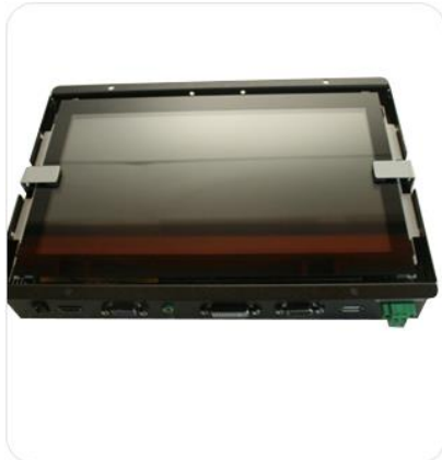
Open Frame Wide 10.1 With Optical Bonding and Touch
