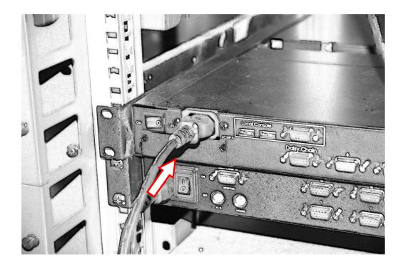
2.5 Connect the host cable to the rear of the drawer. For the BHK117Ue/BHK119Ue, USB type can be connected to its single port. For BHK117-8(16)Ue/BHK119-8(16)Ue both PS/2 and USB type can be use with the KVM, just choose the desire type to match with your system, the KVM accepts both. Refer to **Section 3** for further detail. (\*980 Shown)
