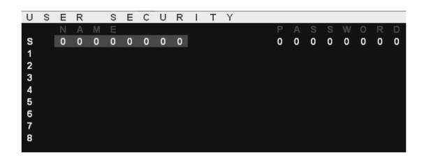
Press the **Enter** key or left button of mouse for editing. The left-top "S" means SUPERVISOR, and "1", "2", "3",..., "8" mean USERs. The maximum length of NAME and PASSWORD is eight characters ( $A \sim Z$  and  $0 \sim 9$ ).
