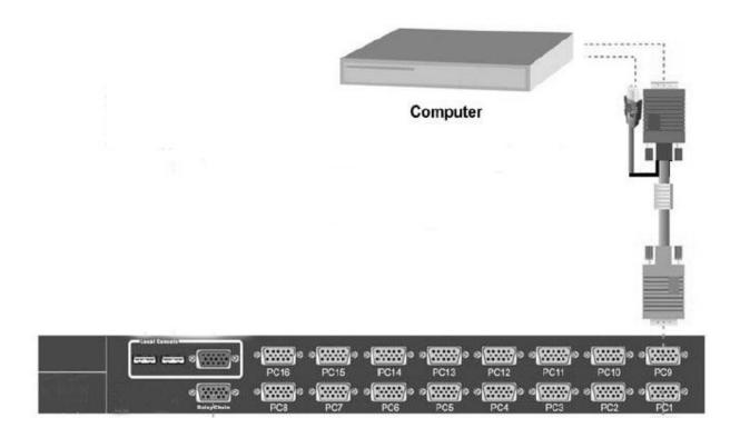
3.4 You can connect a local console port to operate the KVM bypassing the built-in LCD and keyboard/touchpad through the rear local console port. Connect the VGA D-Sub connector and USB keyboard and USB mouse to the port marked.
