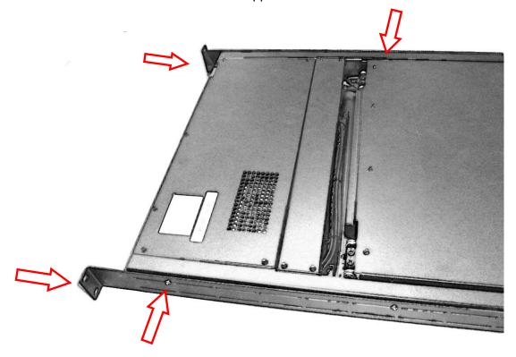
2.3 Secure the rear and front rack mounting to properly mount and fix its position into the cabinet.
