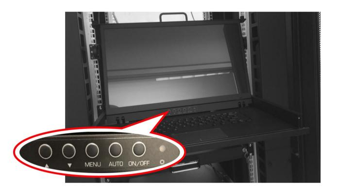
11. To return the drawer back to the unit, fold screen down and push in the 2 taps located on each side of the rail to push the drawer back in.
