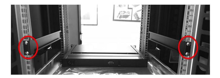
2. After you have mounted the **BHKW117HDe/BHKW117HDUe** Rear Support Brackets into the backside of your rack cabinet, move to the front of your cabinet to slide the **BHKW117HDe/BHKW117HDUe** into the **Rear Support Brackets**.
