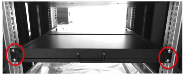
4. Double check and ensure that you have secured the rear and front of the **BHKW117HDe**/ **BHKW117HDUe** onto your rack cabinet properly and fix its position in the cabinet if necessary
