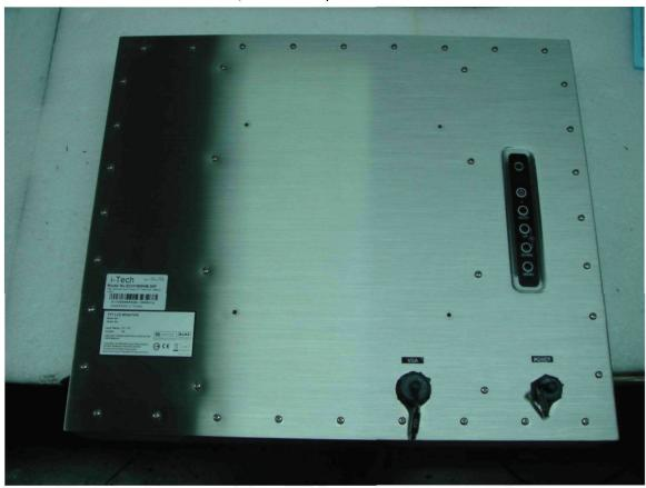
2. Remove internal VGA, OSD keyboard and power input cables to separate back cover from monitor.
