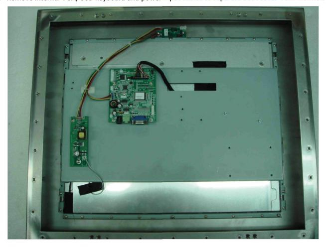
3. Replace backlight controller and OSD keyboard on back cover
