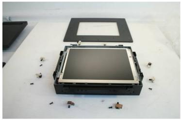
Step 4 - remove 4 screws mark down with red color X, this 4 screws holding LCD panel. See bellow pictures for details.
