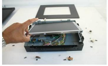
Step 5.- lift up the LCD panel, to access to internal components of the unit. please help us to check all internal connections, inverter board connection, LVDS cable connection to LCD panel, LVDS connection to AtoD board, If everything look fine but still the same issue, we may have to replace the inverter controller board, but please also help to check is when you turn up the unit do you see any backlight on the screen or is completely back screen all the time.
