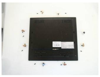
Step 3 - after remove all screws you will be able to remove the front bezel. See bellow pictures for details.
