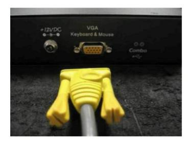
The **yellow** VGA connector is connected to LCD/Keyboard Drawer
